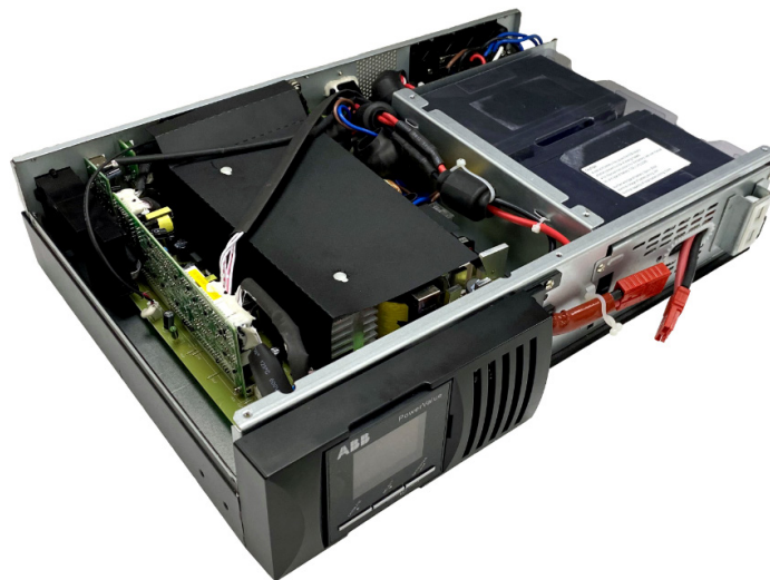
Figure 4-3 PowerValue 11 RT G2, top cover removed
