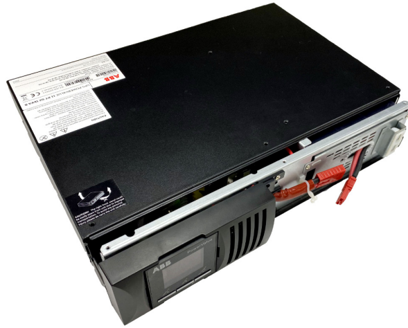
Figure 4-2 PowerValue 11 RT G2, top cover removal
