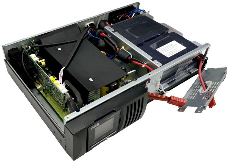
Figure 4-4 PowerValue 11 RT G2, front plate removed
